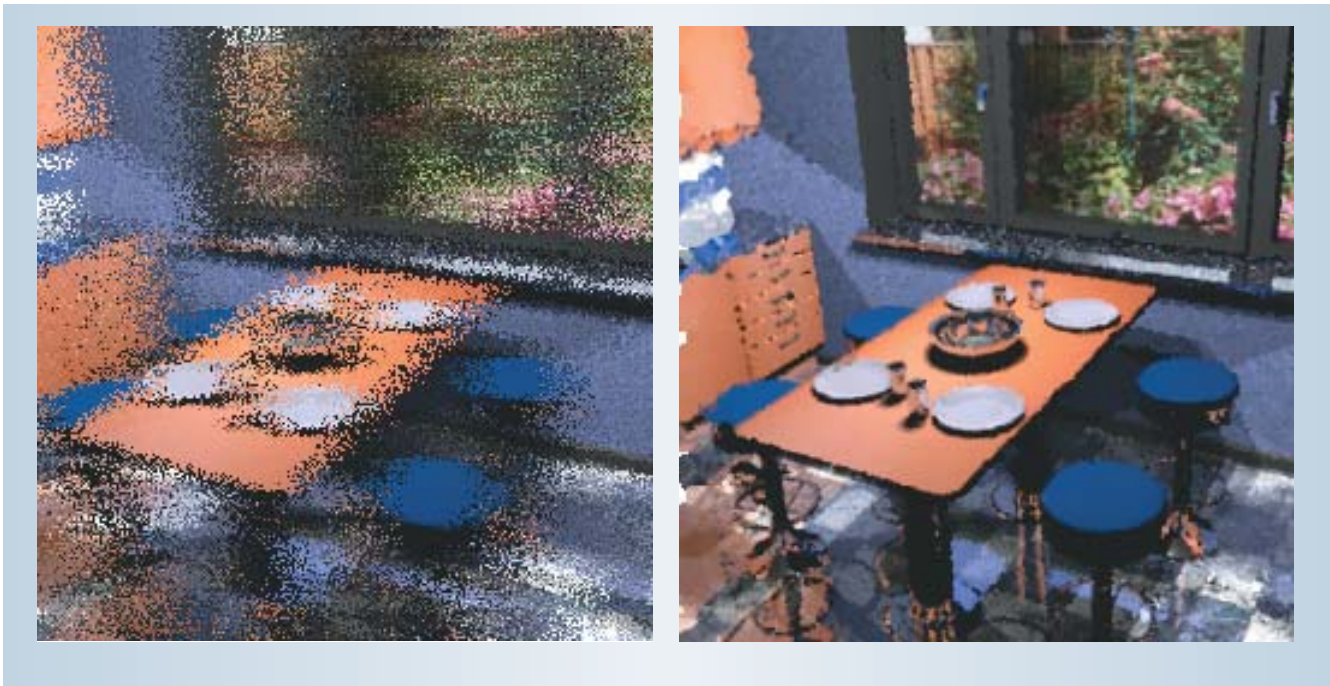
Figure 1. Prototype images showing just adaptive frameless rendering (left) and the result of also applying adaptive reconstruction to these samples (right).
